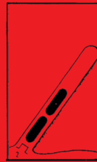
Stage 2 The cartridge or cartridges with a "red cap" are inserted.
