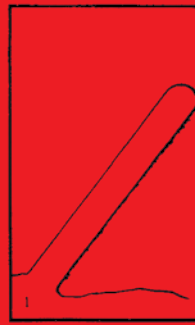
Stage 1 Boreholes of proper depth and diameter are drilled and blown free of dust.
