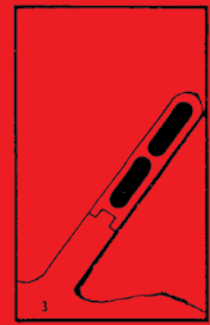
Stage 3 The cartridge or cartridges in position, retained by a "red cap."
